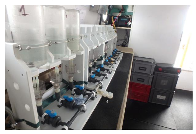
Filtering for total suspended matter with the new filtration manifold that was installed in the wet lab of the *R/V Téthys II*.
